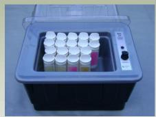
Typical capacity is up to 25 Dipslides or 30 Petri Dishes (95mm)
