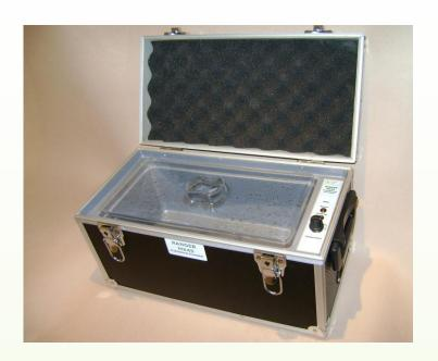
The Ranger MX45 sets new standards for portable incubation of dip slides and other Rapid tests or traditional plates. Designed to be used in the field, site or laboratory and supplied ready for use on mains (worldwide plug & voltages) or 12 volt (vehicle cigar lighter) as standard – all ready to go! Our tested MX solid state temperature control technology and heat reservoir chassis guarantee superb heat distribution without any fans or moving parts.
